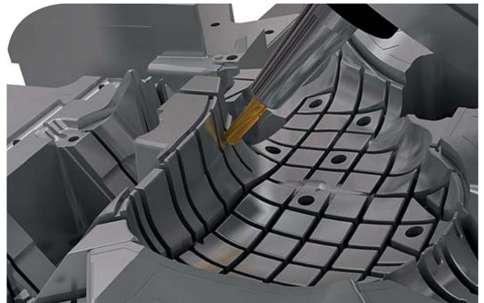
5 axis machining of a mold with TopSolid'Cam.
